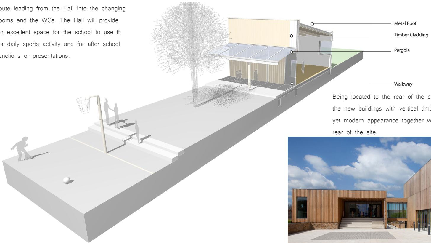
Being located to the rear of the site it is proposed to clad the new buildings with vertical timber slats to create a uniform yet modern appearance together with the other blocks on the rear of the site.
